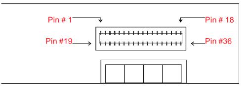
Pins #1 through #16 correspond to outputs #1 through #16 respectively. Pins # 17 through # 36 are circuit common.
